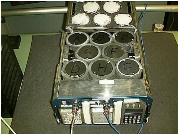
Figure 7. CGBA-03 Payload with Temperature Controlled Containers
